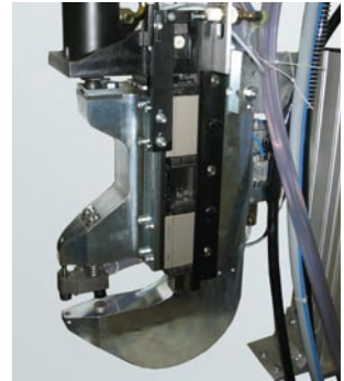
C-frame for difficult to access areas e.g. wheel house
