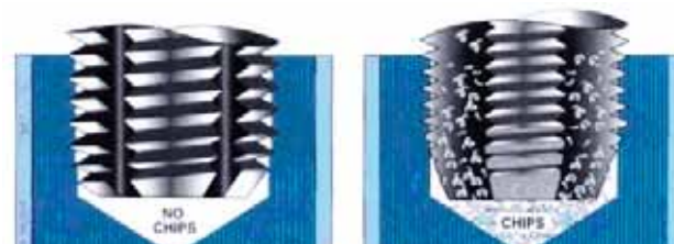
Forming tap with oil grooves
