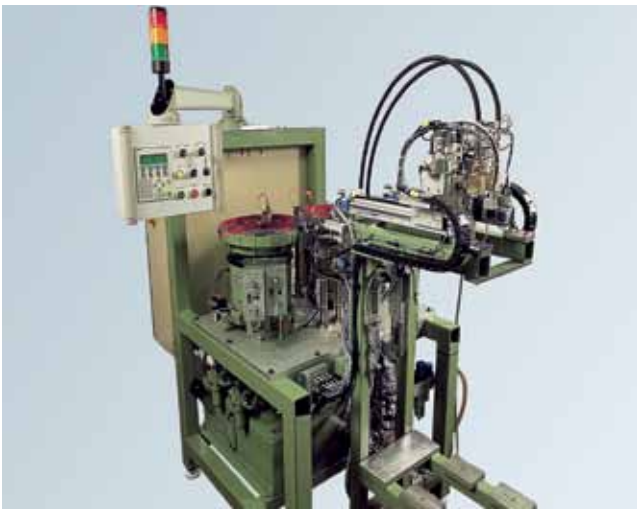
MIRS System to assemble vacuum pump
