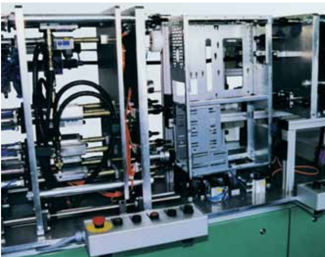
29 placing heads to assemble computer chassis
