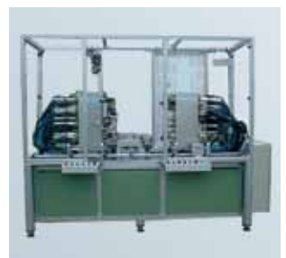
23 placing heads to assemble a computer chassis
