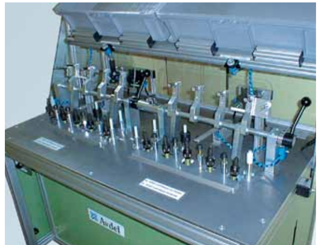
10 placing heads to assemble automotive sealing strips
